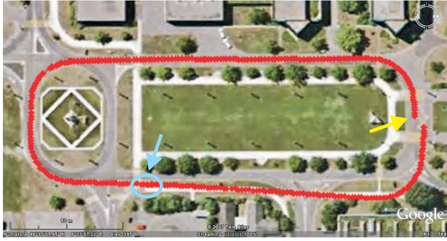
Fig. 6. The estimated path (before loop closing) superimposed onto a Google Earth image of the test environment. The scale is shown at the lower left corner.
