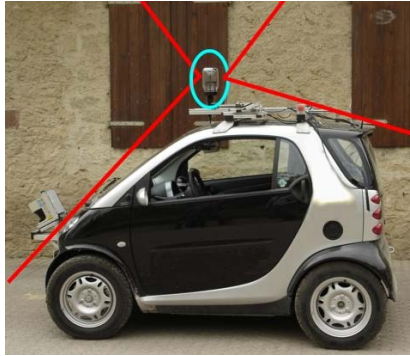
Fig. 1. Our vehicle with the omnidirectional camera (blue circle). The field of view is indicated by the red lines.
