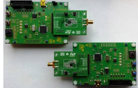
Figure 3. STMicroelectronics STEVAL-IKR002V5 boards.
