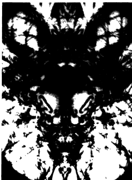
Fig. 10. — Tanaka pattern along [110] of a vertical coherent twin boundary in Si. The trace of the boundary plane runs vertically through the centre of the pattern (from Ref. [11]).
