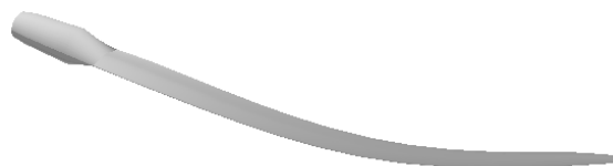
Figure 7: Blade flapwise deflection
