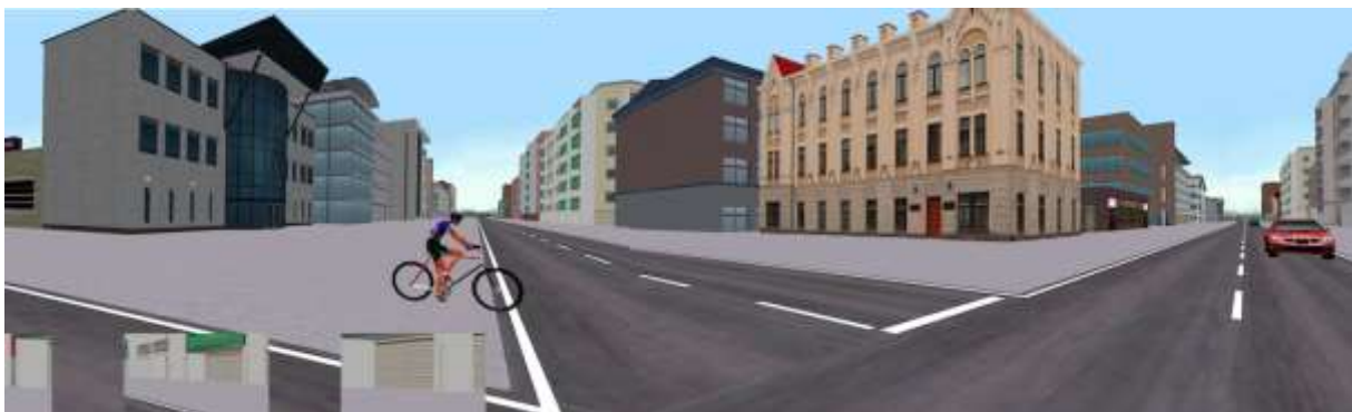
Figure 21: Cyclist stops at road-side, but system still activates ('false positive'). Note: image is slightly distorted due to projection on an immersive, wrap-around screen; road turning is actually at 90° to main road.
