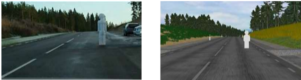
Figure 30: Test Track and Virtual world, critical object spawn position.
