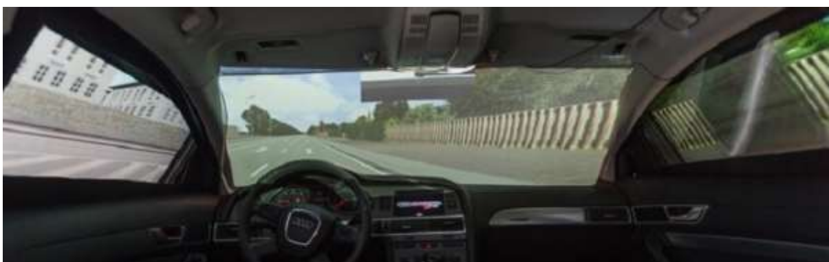
Figure 12: The Vehicle in the loop system used for TME study
