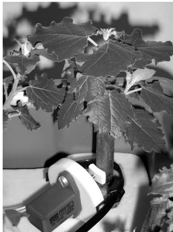
Fig. 1. Radial growth measured with a linear motion sensor on the stem of Populus tremula × Populus alba clone 717-1B4 cultivated under hydroponic conditions.
