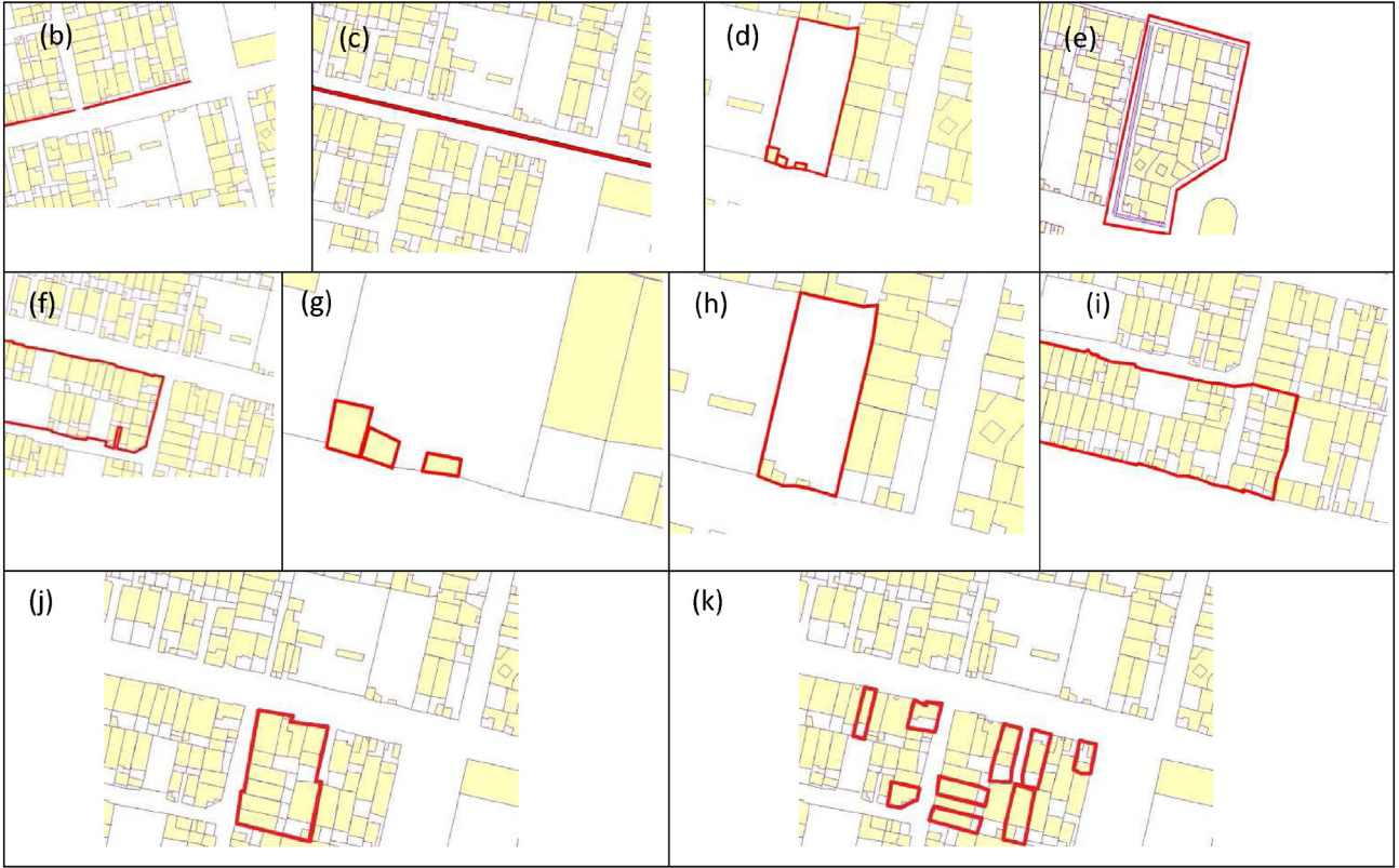
Fig. 3. (a) The ontology of the urban environment layouts describing the components of a city and an illustration of (b) edge, (c) path, (d) parcel, (e) urban area, (f) block (isolated parcels), (g) building lot, (h) parcel boundary, (i) district (parcel set), (j) parcel set (parcels with connections to others) and (k) parcel set (separated parcels).
