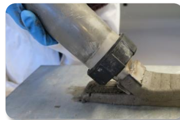
Fig. 3: Extrudability test
