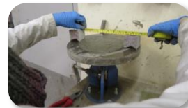
Fig. 2: Slump flow test
