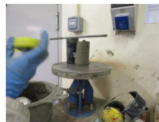
Fig. 4: Slump of cylinder test
